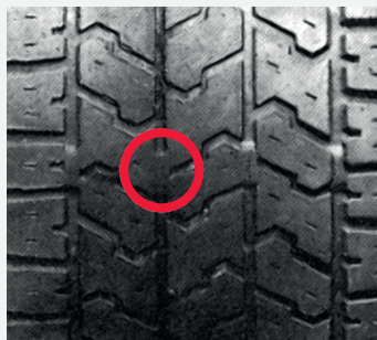
The TWI (1,6 mm): is equal to the tread
